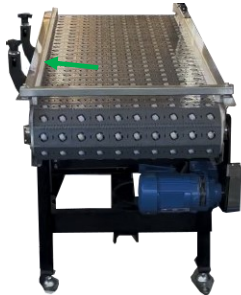
30deg angled roller top for box positioning
