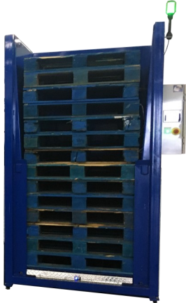
Pallet dispenser - for GMA or CHEP 48 x 40 pallets. (Custom designs available)
