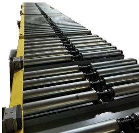
45deg angled roller top 90 deg box transfer up to 30 cases / minute
