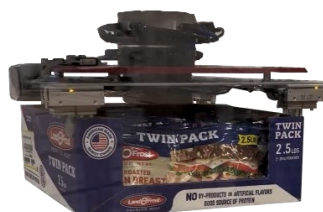
Tray clamping gripper handles up to 35 lbs
