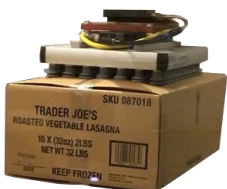
1 box vacuum gripper handles up to 50 lbs
