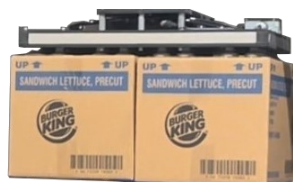
2 box vacuum gripper handles up to 100 lbs
