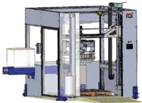
1-Station POD with Stretch Wrapper, 5.5 ft stack height
